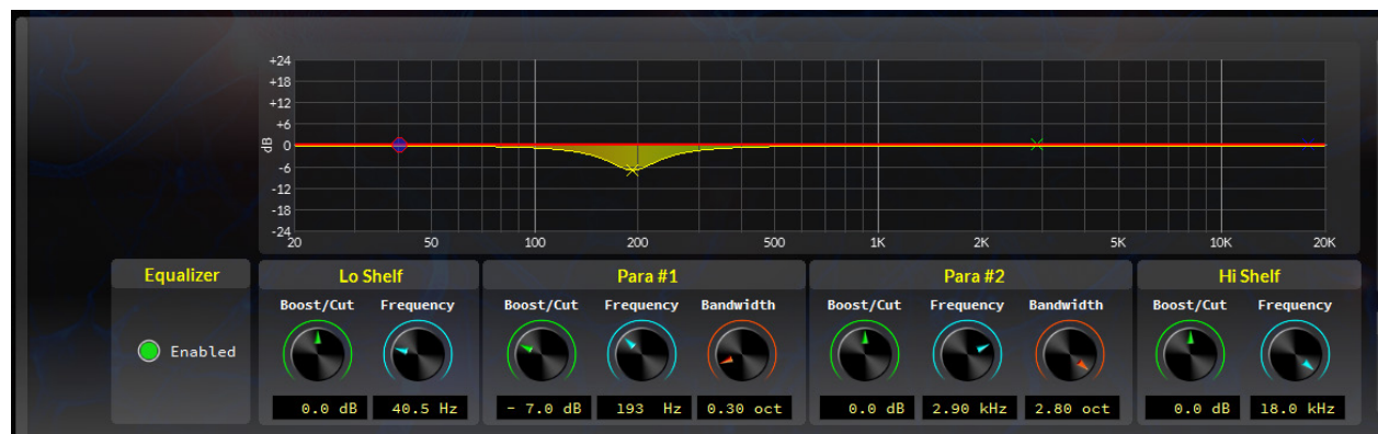
The equalizer is equipped with two parametric equalizers and two shelving filters.
