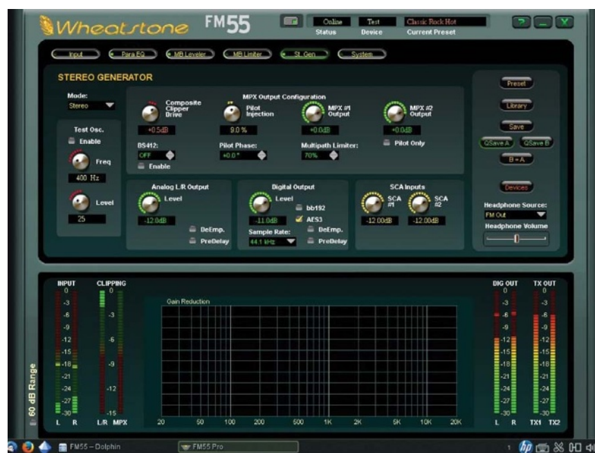
Fig. 3: The Multipath Limiter intelligently controls the L-R energy.
