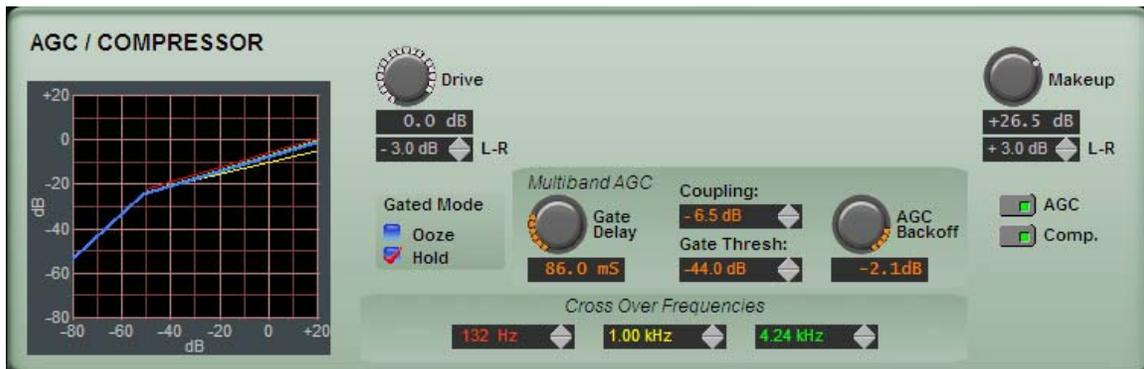
The individual adjustments for each band's attack and release times, compression ratios, and band gate thresholds, etc. are shown by the blue dots on the graphic below.
