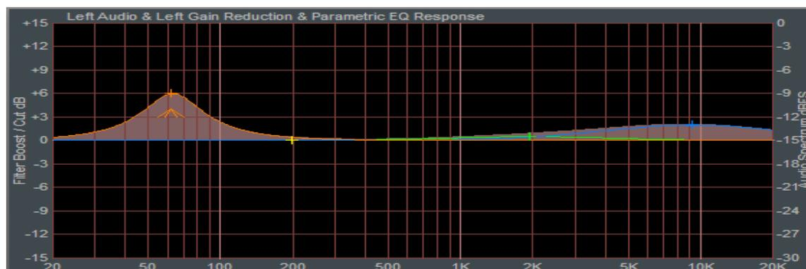
The VP8's parametric equalizer is an especially effective tool for sweetening voice. In the curve shown on the previous page we've adjusted it to warm up the sound of a popular mid-priced microphone by increasing the amount of energy at the lower extremes of male voice while also giving it a bit of 'air' by slightly increasing the gain near 9kHz.
