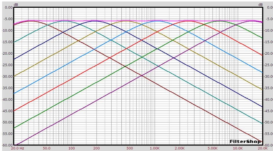
The most important thing to recognize is how broad the crossovers actually are in the eight band example – and the typical four or five band crossover *could* be even broader depending on its design.
