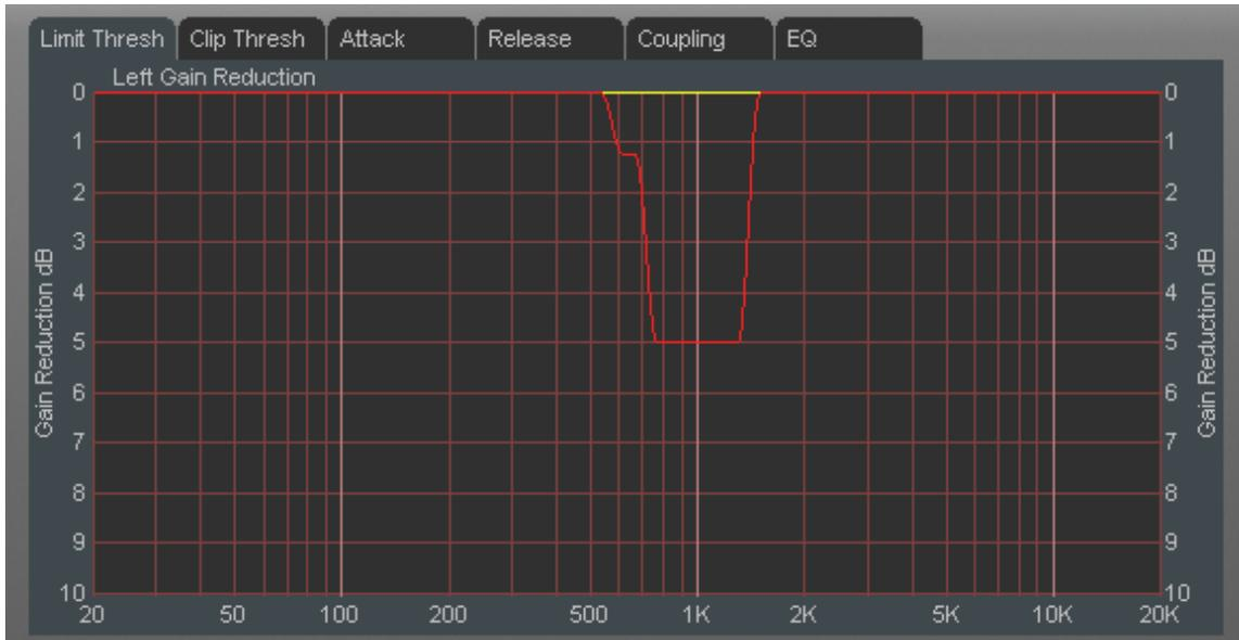
Notice how the range of the frequencies undergoing limiting is wider than in the first example? This is because there are now three bands in limiting even though the 1 kHz tone is present at the center of only the middle band.
