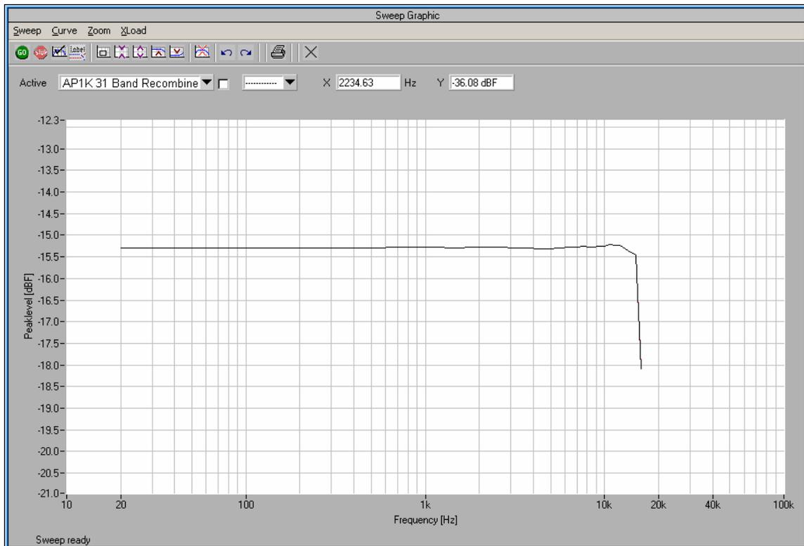
As can be seen from the plot, other than some expected amplitude ripple just prior to the abrupt cutoff of the 15 kHz FM low pass filter the recombined frequency response is virtually flat. And like the frequency response, the phase linearity is also flat with no abrupt departures from linear phase.
