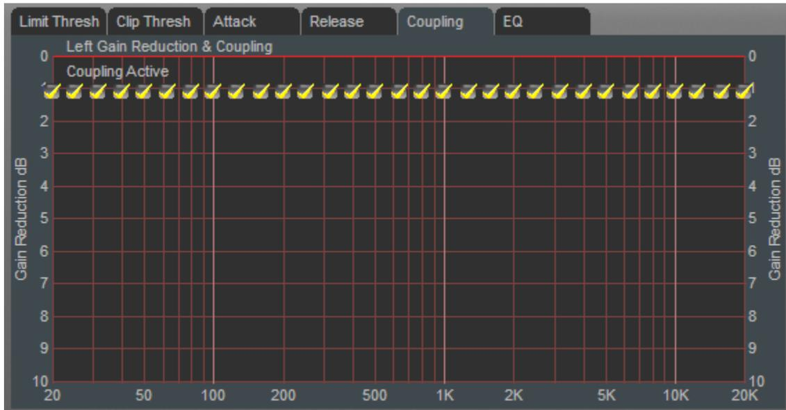
The Coupling controls in the 31 band structure don't couple the control signals from one band to another as is common for the term "coupling", the controls 'hook' or 'unhook' a band from the Wide or Timbral mode when it is running. You cannot unhook a band from Discrete mode!
