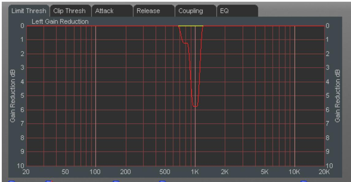
Because there is no limiting at any frequency other than what is required by the 1 kHz tone, any program material that would be near 1 kHz but not high enough to cause its own limiting activity would remain at its original amplitude!
