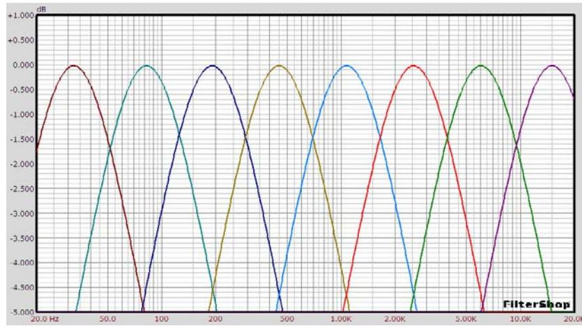
Compare this to the plot below – which is an example of the type of filter bank used in the AP2000 (limited here to just sixteen bands to keep the graphic image clearer).
