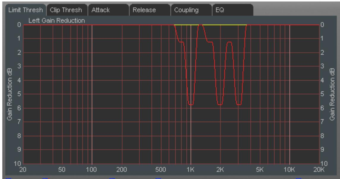
Notice how the 1 kHz band is still in 6dB of limiting but now there is also 6dB of gain reduction occurring in the 2 kHz and 3 kHz bands? This is precisely what the Timbral Mode does – it calculates the harmonics of the primary signal requiring limiting and causes *equal* gain reduction at that frequency as well as its second *and* third harmonics.
