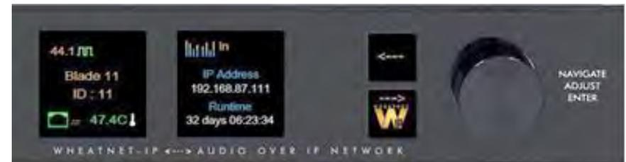
**Figure 3-3 Mix Engine Front Controls, System Info Displays**
