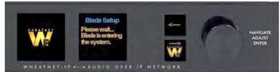
**Figure 3-2 Mix Engine Front Controls, Entering the System**
