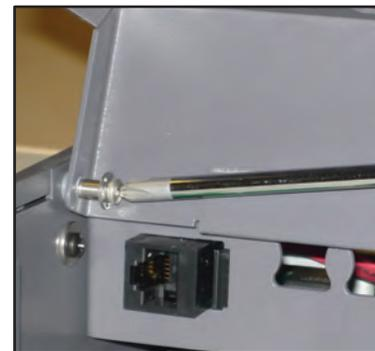
Removing the Rear Cover Left Hinge Screw
