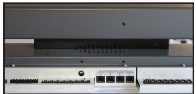
DIRECT VIEW METER MOUNTING SCREWS
